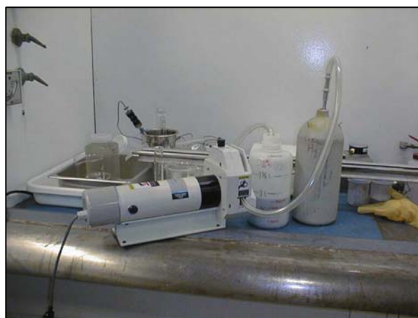
Figure 34. A peristaltic pump will be used for transferring mercury.
